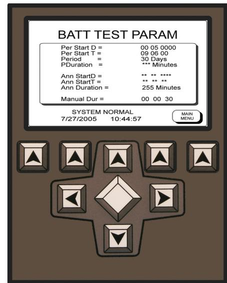
The LCD display on the model **"ELE" Intellistat** provides all electrical parameters, inverter status, programmable inverter and battery testing, remote monitoring and reporting, and data logging. An optional integrated fax modem can be included in the closed-loop communications system.
